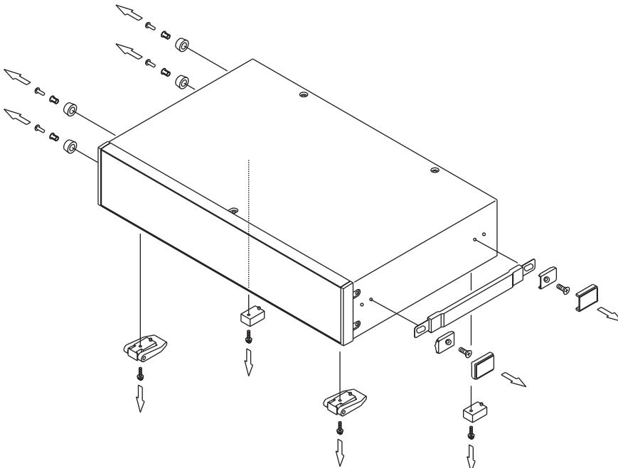
2. As shown in figure, using the accompanying screws, install the brackets. Do not use except the accompanying screws (M3 x 10).
