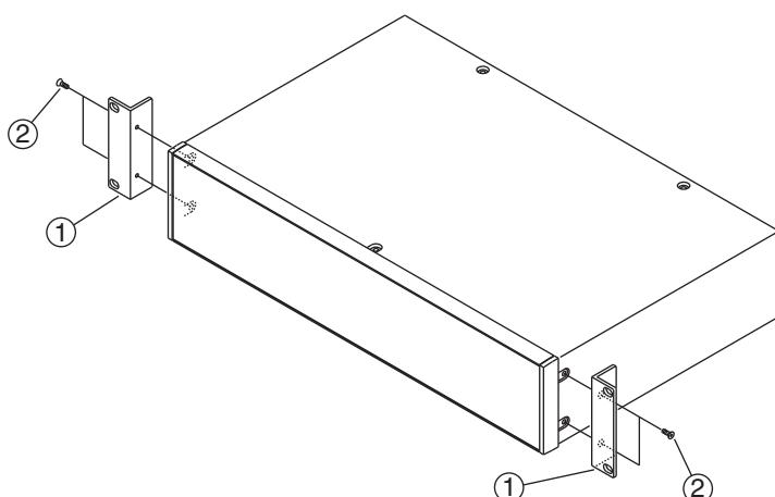
3. Using the accompanying screws and washers, mount the instrument in the rack.
